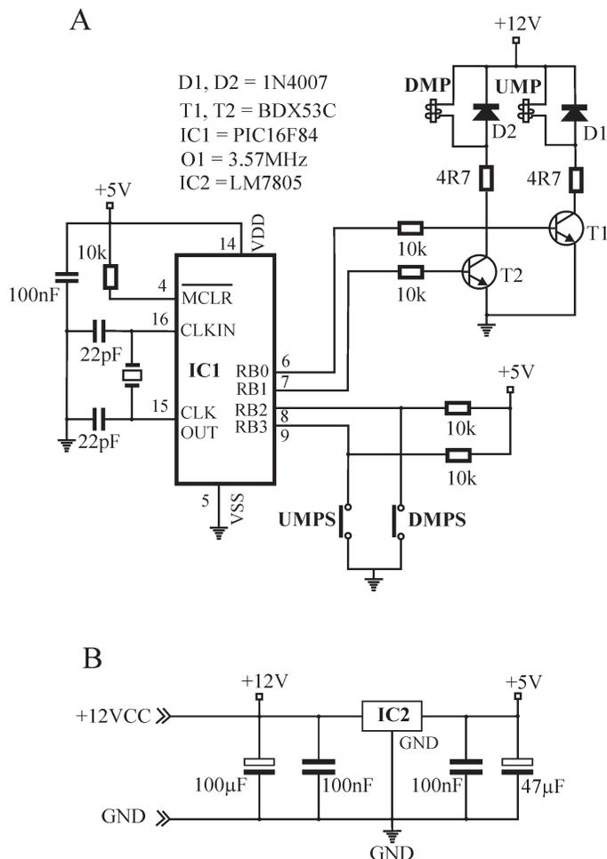
**Fig. 3.** Schematic diagram of the electronic switching system. A is microcontroller and B is power supply regulator. DMP, downward moving pump; UMP, upward moving pump; DMPS, switch of the downward moving pump; UMPS, switch of the upward moving pump.
