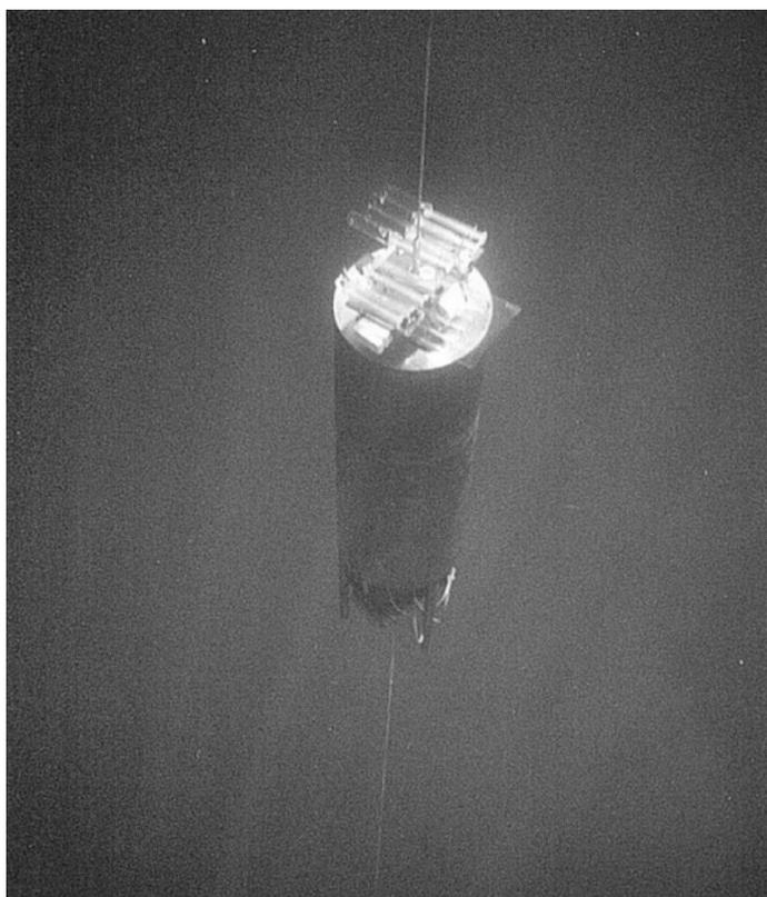
**Fig. 4.** Picture showing the MIRI during its operation in Lago Moreno waters, carrying a frame holding the incubation tubes. The top of the cylindrical buoy was made white for visibility.
