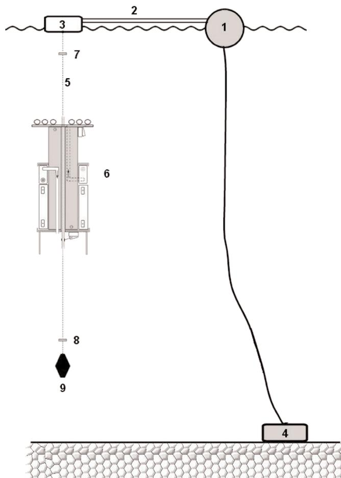
**Fig. 2.** Mooring of the instrument. 1, main floater; 2, rigid connection; 3, transparent buoy; 4, anchor weight; 5, driving rope; 6, MIRI; upper (7) and lower (8) run limiters; 9, MIRI driving rope weight.
